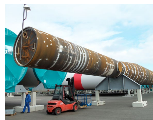
Monopile foundation of a met mast.
